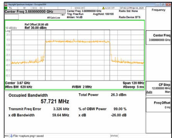
n48 60M DFT-s-OFDM 64QAM Outer_Full High
