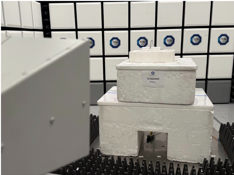
Figure 4 Antenna Pattern Test at 3 meters (Front view)
