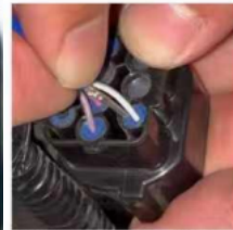
Yellow : Turn left to positive, blue : turn right to positive
