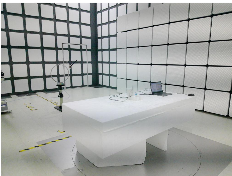
Description: Radiated Emission Test Setup for 9kHz~30MHz
