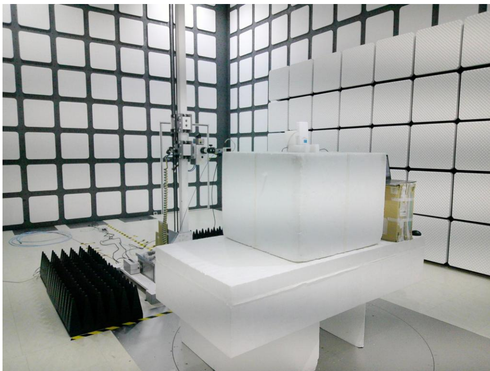
Description: Radiated Emission Test Setup for 9kHz~30MHz
