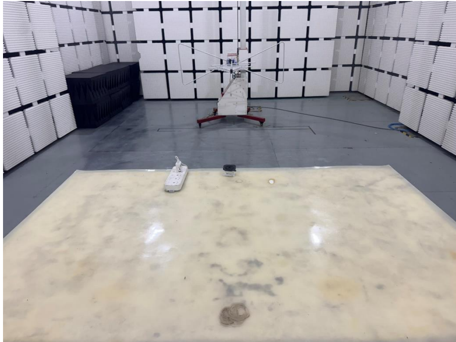
Set-up for Radiated Spurious Emission, Above 1GHz
