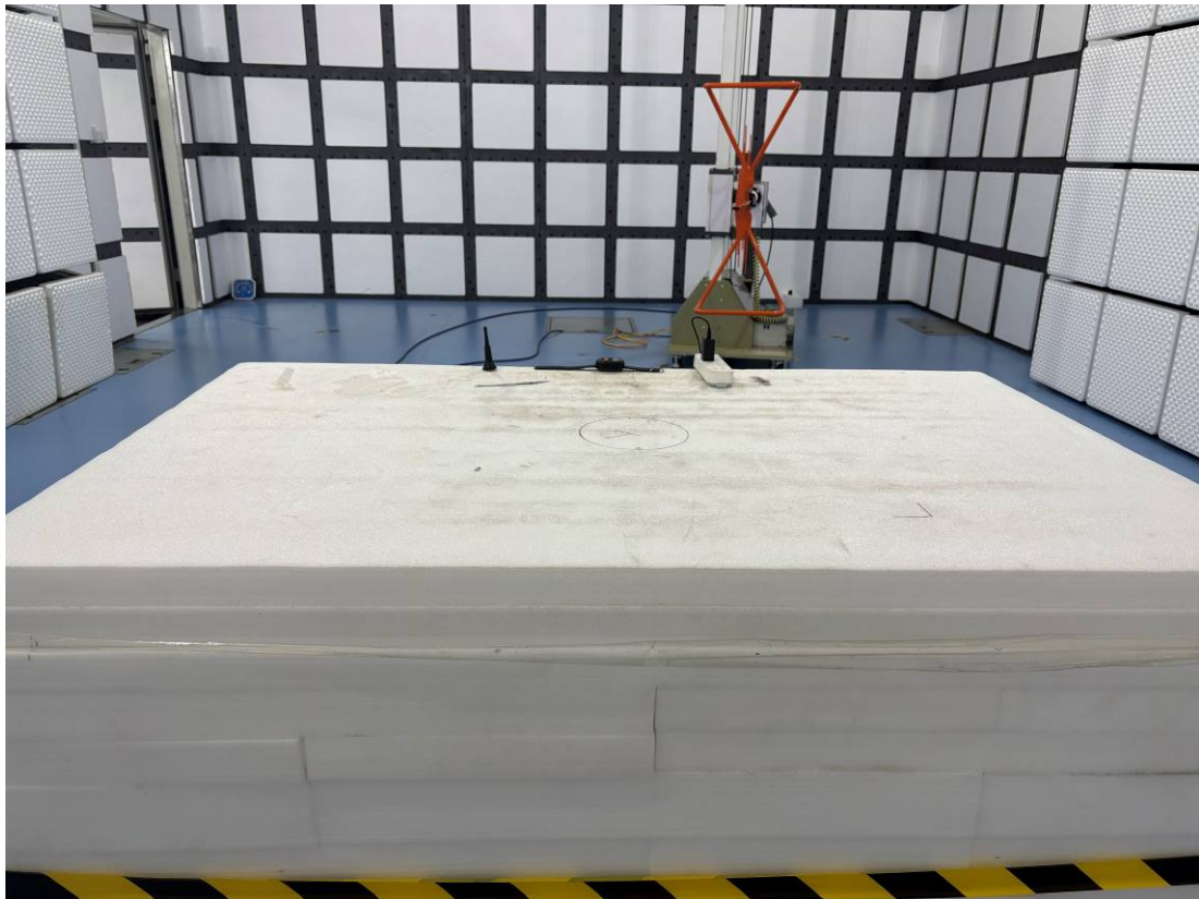
Radiation Emission - Back View (Below 1GHz)
