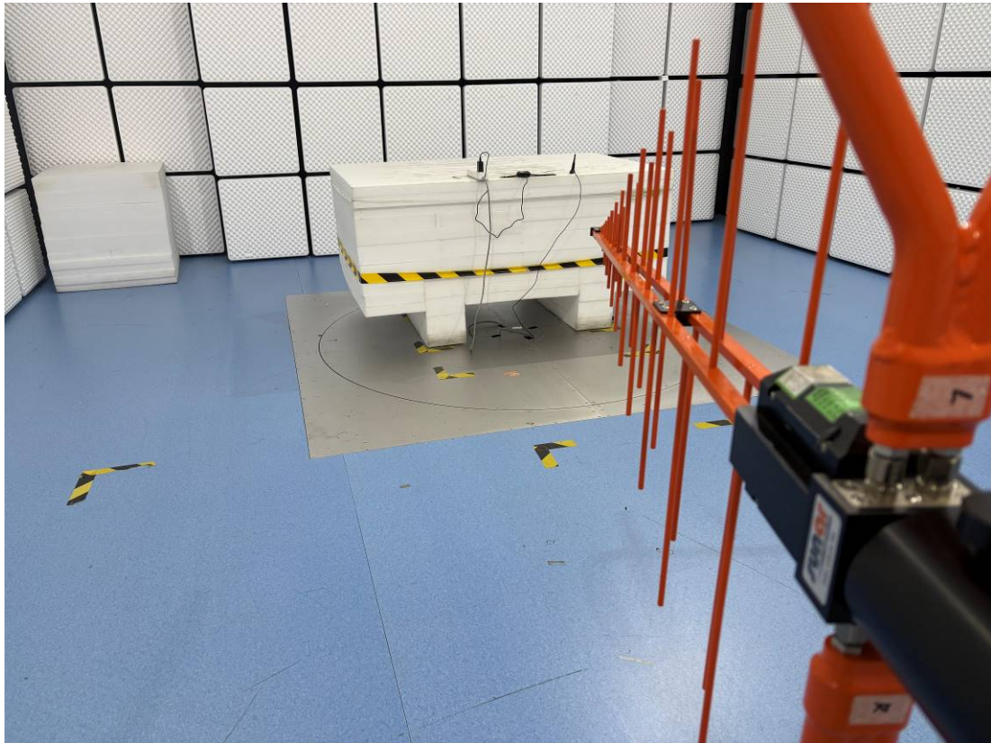
Radiation Emission - Back View (Below 1GHz)
