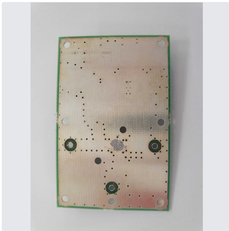
Photo 19 RF Switch Board bottom
