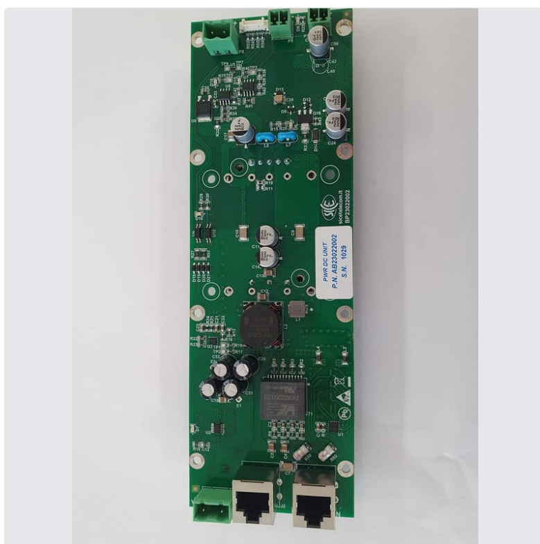
Photo 16 Power Supply Board top
