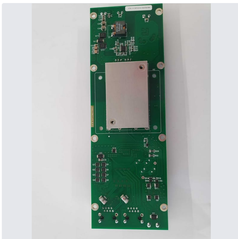
Photo 15 Power Supply Board bottom
