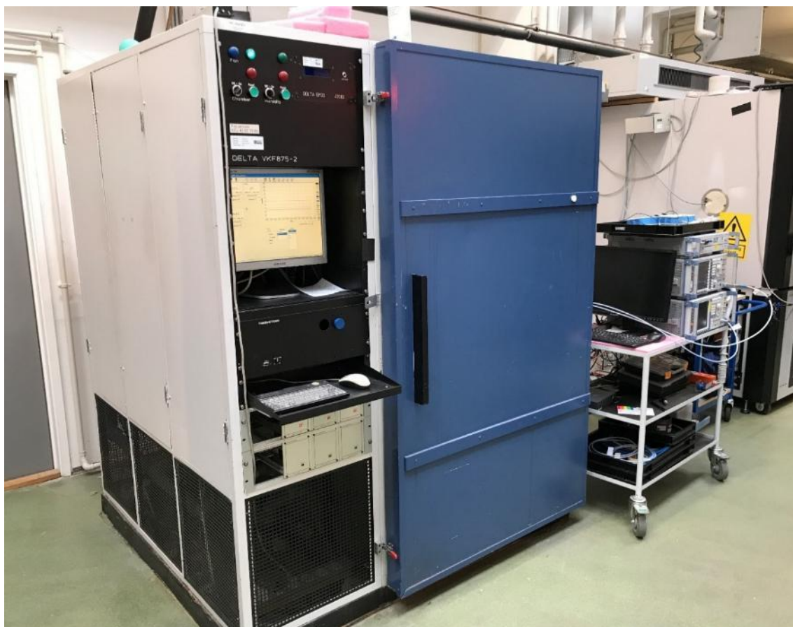
Photo 4.5.3 Measurement of frequency stability with respect to ambient
