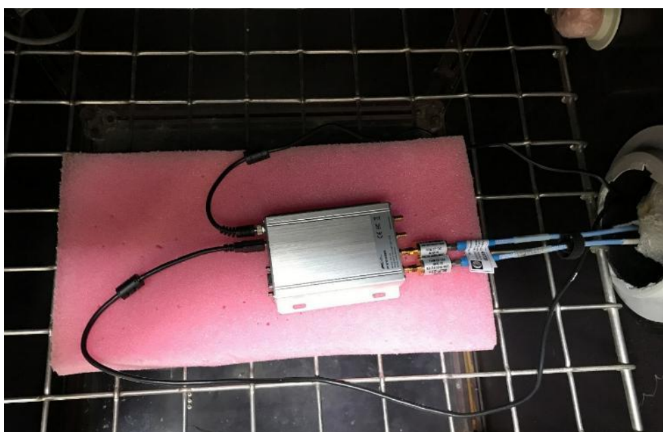
Photo 4.5.2 Measurement of frequency stability with respect to ambient
