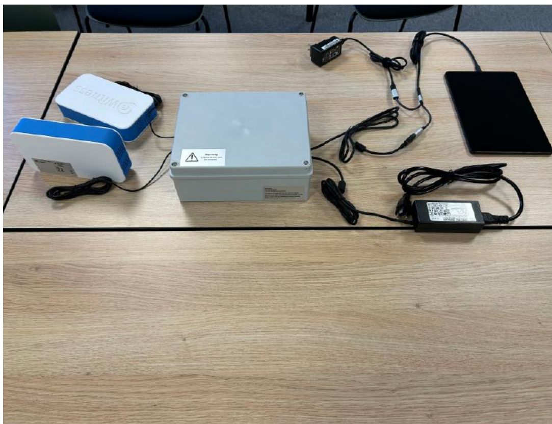
Photo 1.1.10 - Test item 2 placed in the final enclosure
