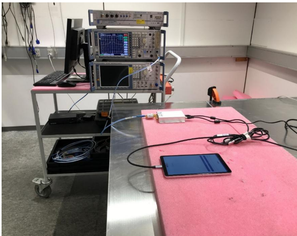
Photo 4.5.1 Measurement of frequency stability when varying supply voltage
