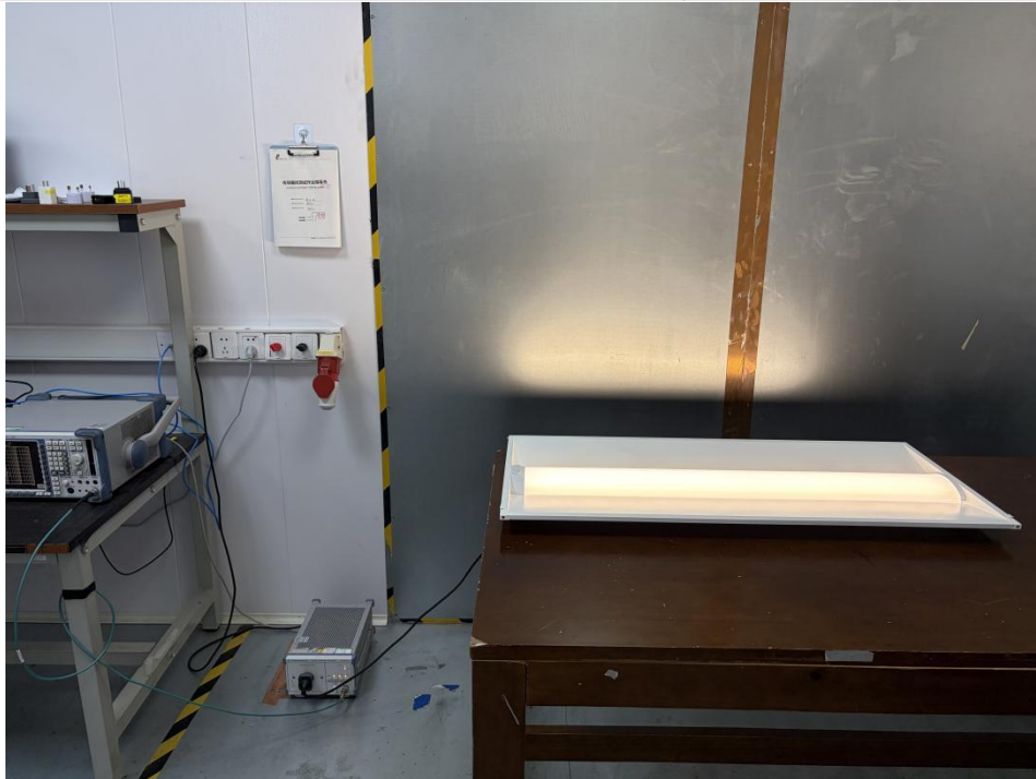
Conducted emissions at AC power line (150kHz-30MHz)
