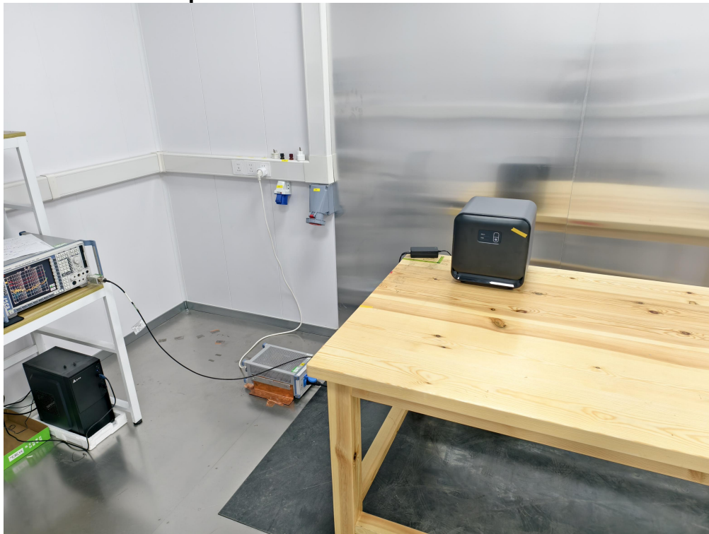
Photo 3 Test Setup Photos of AC Power Line Conducted Emissions
