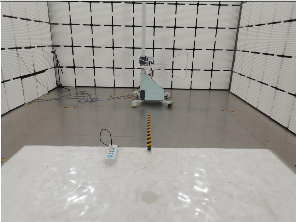
Radiated Spurious Emission, Below 1GHz
