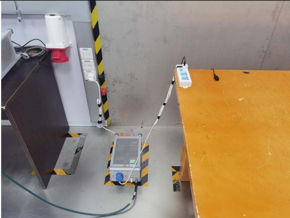
Radiated Spurious Emission, Below 1GHz
