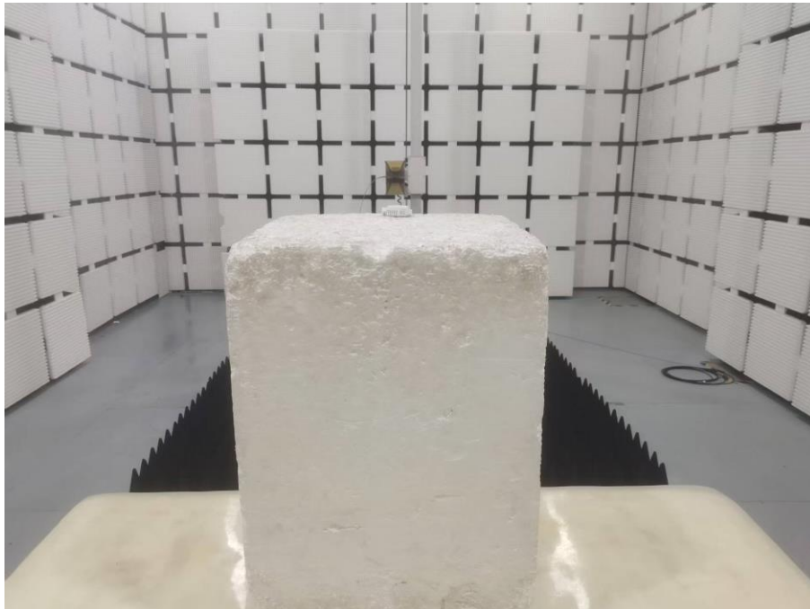
Set-up for Radiated Spurious Emission, Above 1GHz
