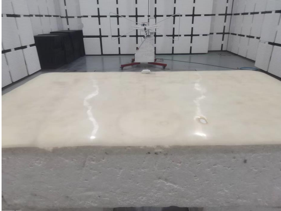
Set-up for Radiated Spurious Emission, Above 1GHz
