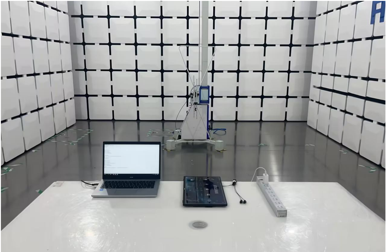
Radiated Spurious Emission Test View 1
