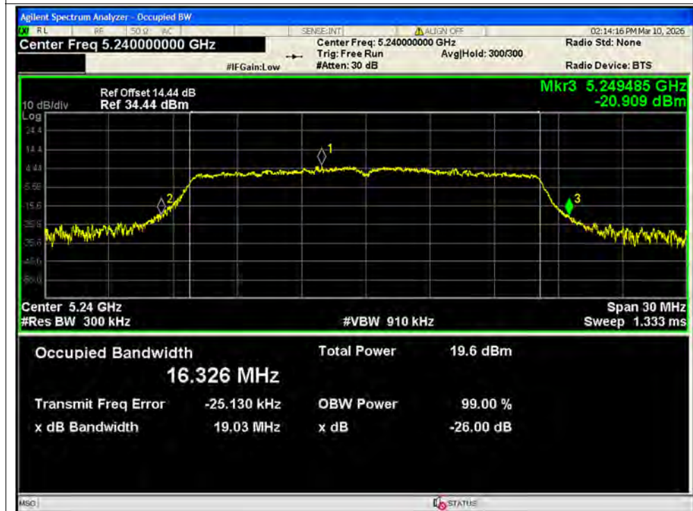
-26dB Bandwidth NVNT a 5240MHz Ant2 SISO
