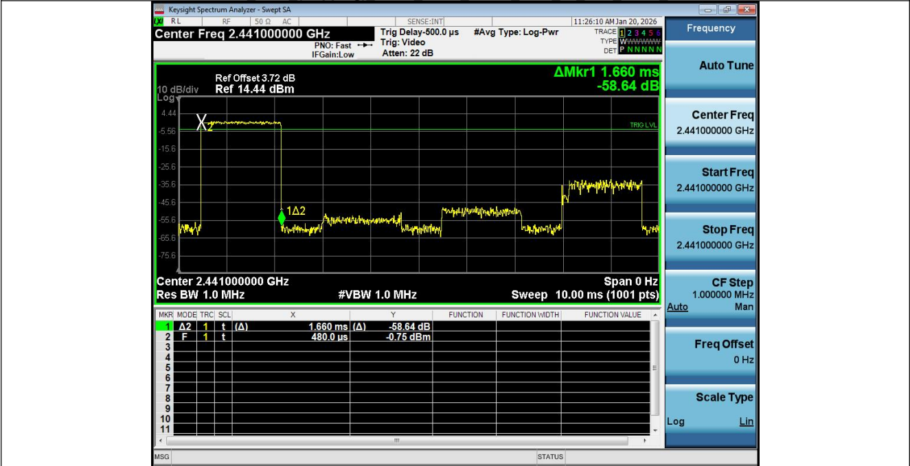
Dwell Time (Hopping) NVNT_ANT1_3-DH3_2441_00_Accumulated
