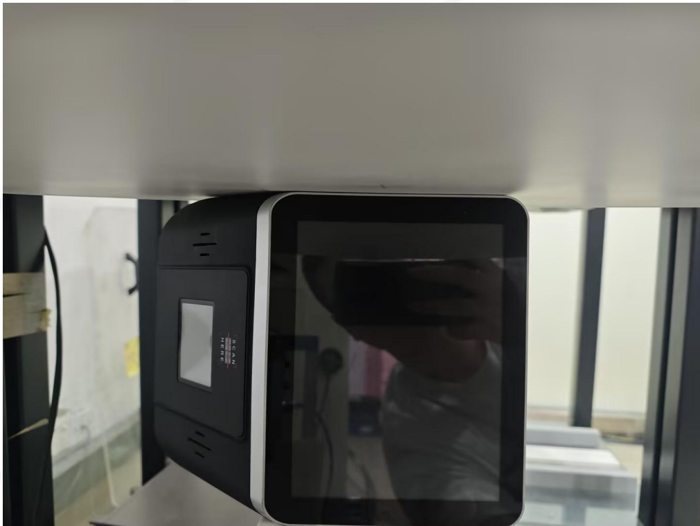
Body Left Edge (separation distance is 0mm)
