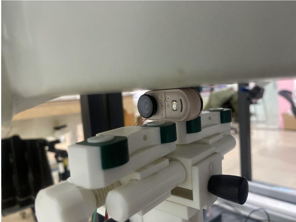
Body Right Side (separation distance is 0mm)
