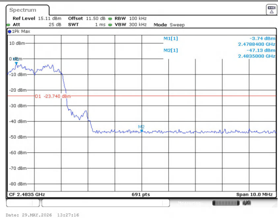
Out Of Band Emission(Right) 8DPSK_3-DH5_Channel Hopping
