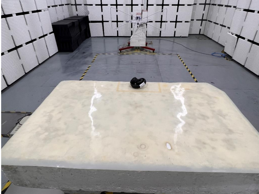
Set-up for Radiated Spurious Emission, Above 1GHz
