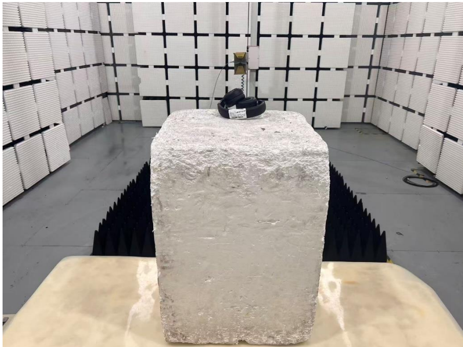
Set-up for Radiated Spurious Emission, Above 1GHz
