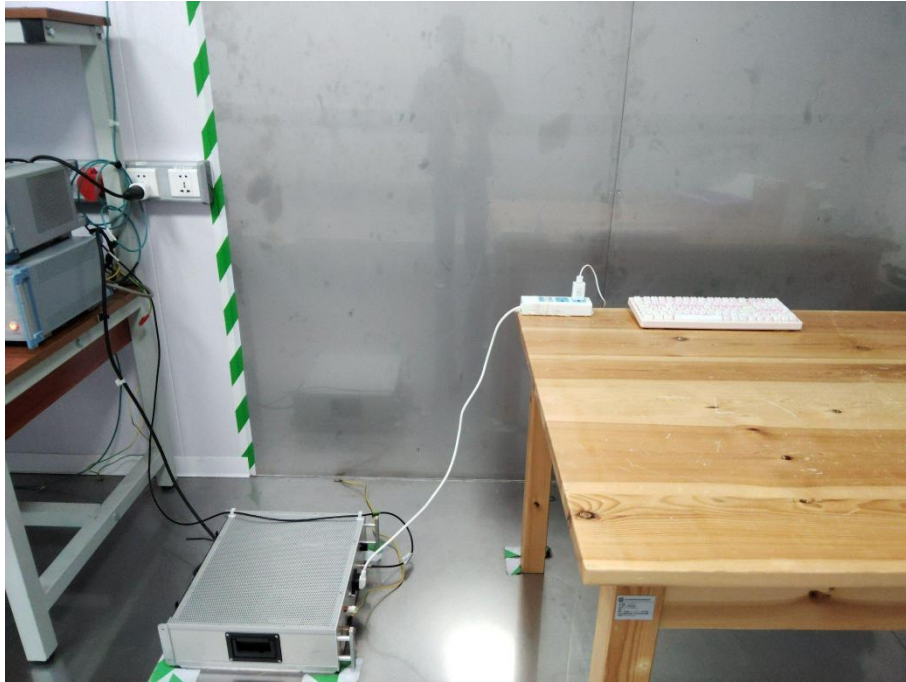
Conducted Emission at AC power line
