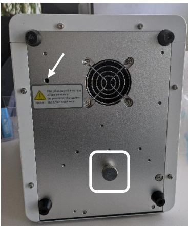
Figure 18. Location of the transport lock screw (highlighted by a white frame) and the storage position (highlighted by a white arrow) on the underside of the QIAmini.
