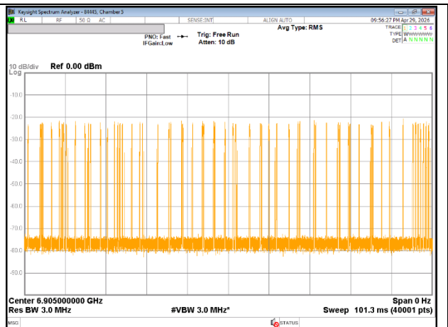
EUT TRAFFIC WITHOUT INCUMBENT SIGNAL PRESENT
