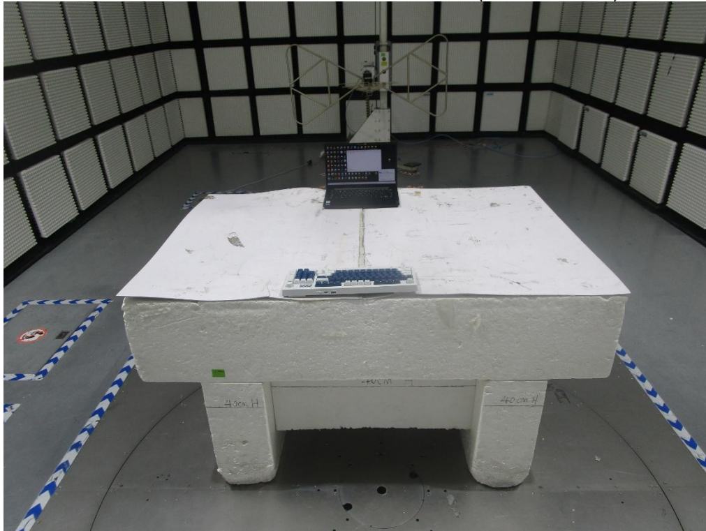
RADIATED RF MEASUREMENT SETUP (Below 30MHz)
