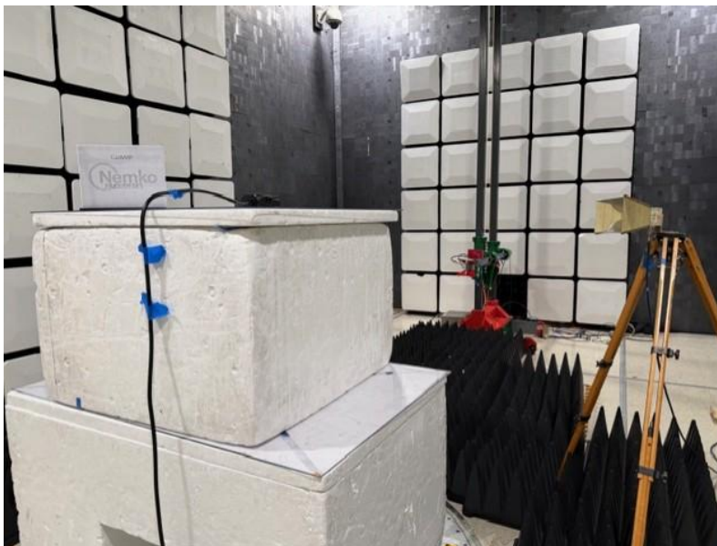
Figure 8.1-10: Radiated emissions setup for 1-18 GHz, BLE+LTE coexistence test (rear view)
