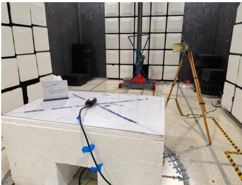
Figure 8.1-8: Radiated emissions setup for 30MHz-1GHz, BLE + LTE coexistence test (rear view)
