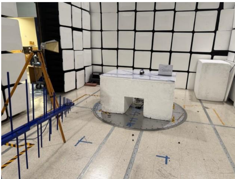
Figure 8.1-9: Radiated emissions setup for 30MHz-1GHz, BLE+LTE coexistence test (front view)
