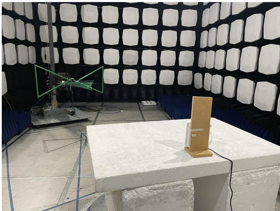
Figure:4 – Test Set up – Rear View of the EUT - Radiated Emissions <1 GHz
