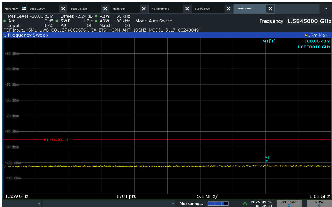
Plot 7-13. Radiated Spurious Emission 1559-1610MHz (Ch. 9, Config 1, Payload 125B Ant. Pol. H)
