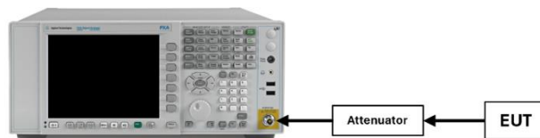
Figure 7-3. Test Instrument & Measurement Setup
