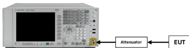
Figure 7-1. Test Instrument & Measurement Setup
