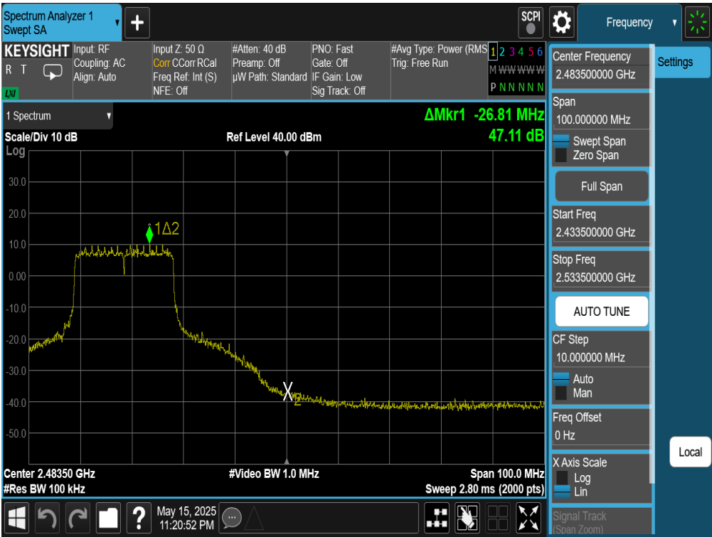
Plot 7-136. Band Edge Plot Antenna WF7 (802.11be (SU - 2.4GHz) – Ch. 9)
