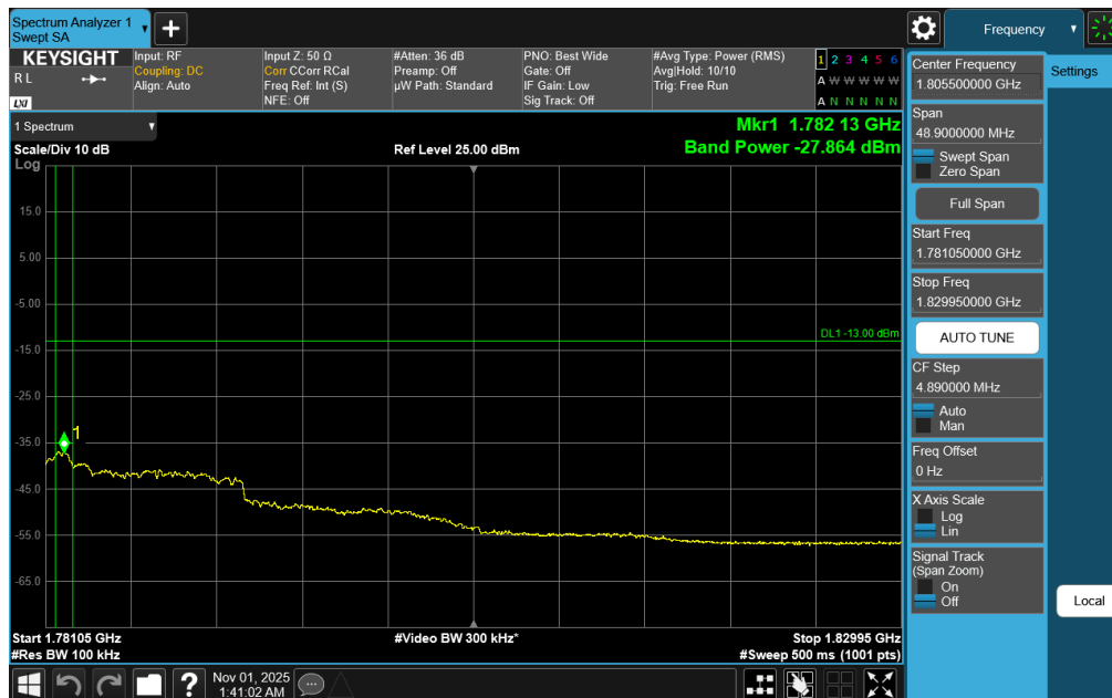
Plot 7-328. Upper Extended Band Edge Plot (NR Band n66 – 15.0MHz DFT-s-OFDM QPSK - Full RB)
