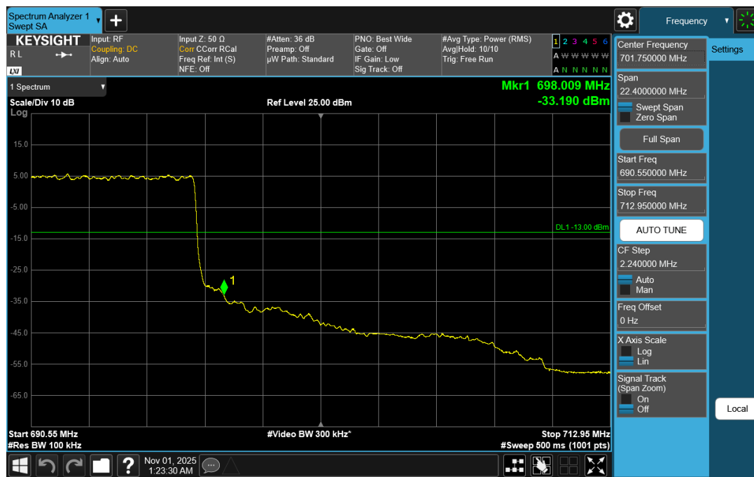
Plot 7-370. Upper Band Edge Plot (NR Band n71 – 15.0MHz DFT-s-OFDM QPSK - Full RB)
