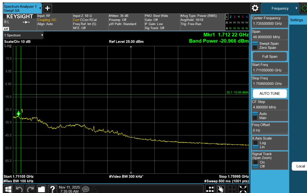
Plot 7-360. Upper Extended Band Edge Plot (NR Band n70 – 10.0MHz DFT-s-OFDM QPSK - Full RB)
