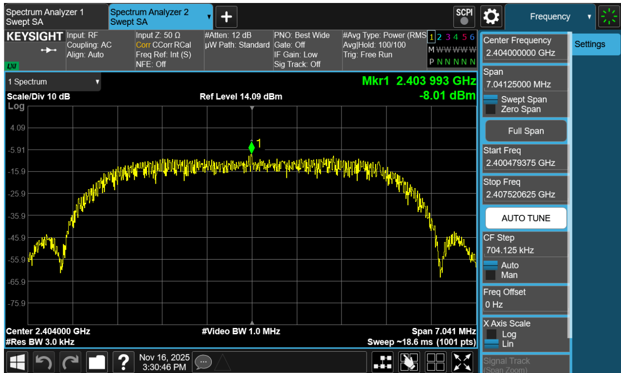
Plot 7-193. Power Spectral Density Plot TxBF Antenna 3a (Bluetooth (HDRPM16), 16Mbps, ePA – Ch. 1)
