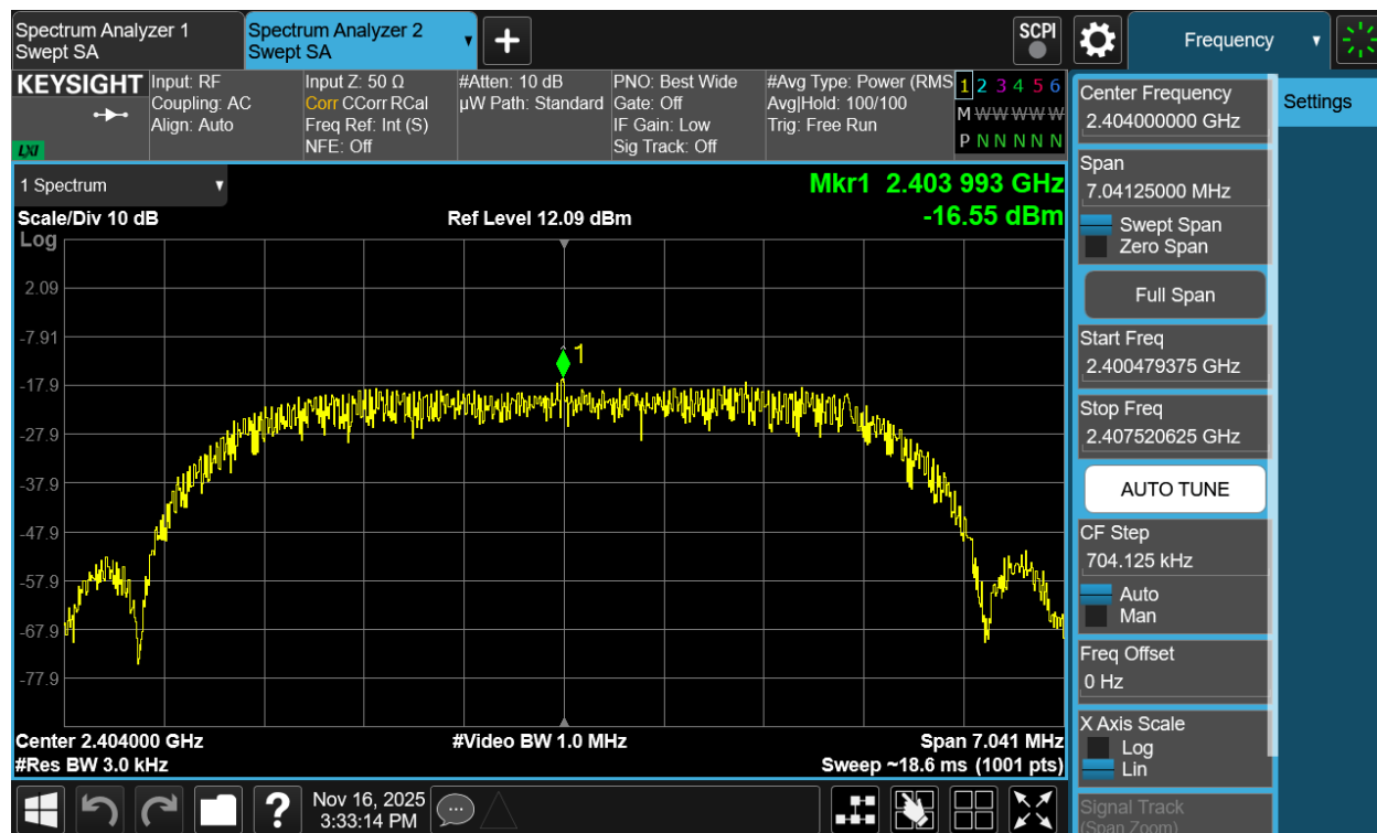
Plot 7-199. Power Spectral Density Plot TxBF Antenna 3a (Bluetooth (HDRPM16), 16Mbps, iPA – Ch. 1)
