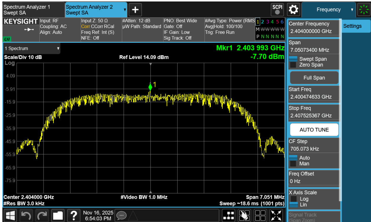
Plot 7-194. Power Spectral Density Plot TxBF Antenna 1a (Bluetooth (HDRPM16), 16Mbps, ePA – Ch. 1)
