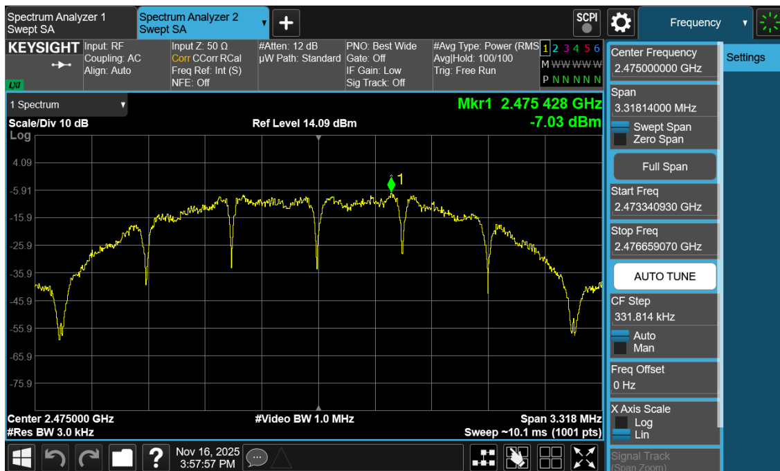
Plot 7-24. Power Spectral Density Antenna 1a (802.15.4, iPA – Ch. 25)
