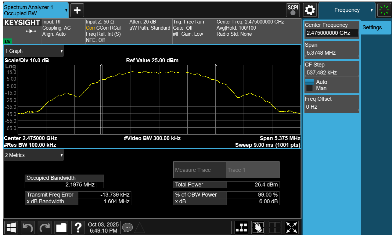
Plot 7-9. 6dB BW Antenna 3a (802.15.4, Ch. 25)
