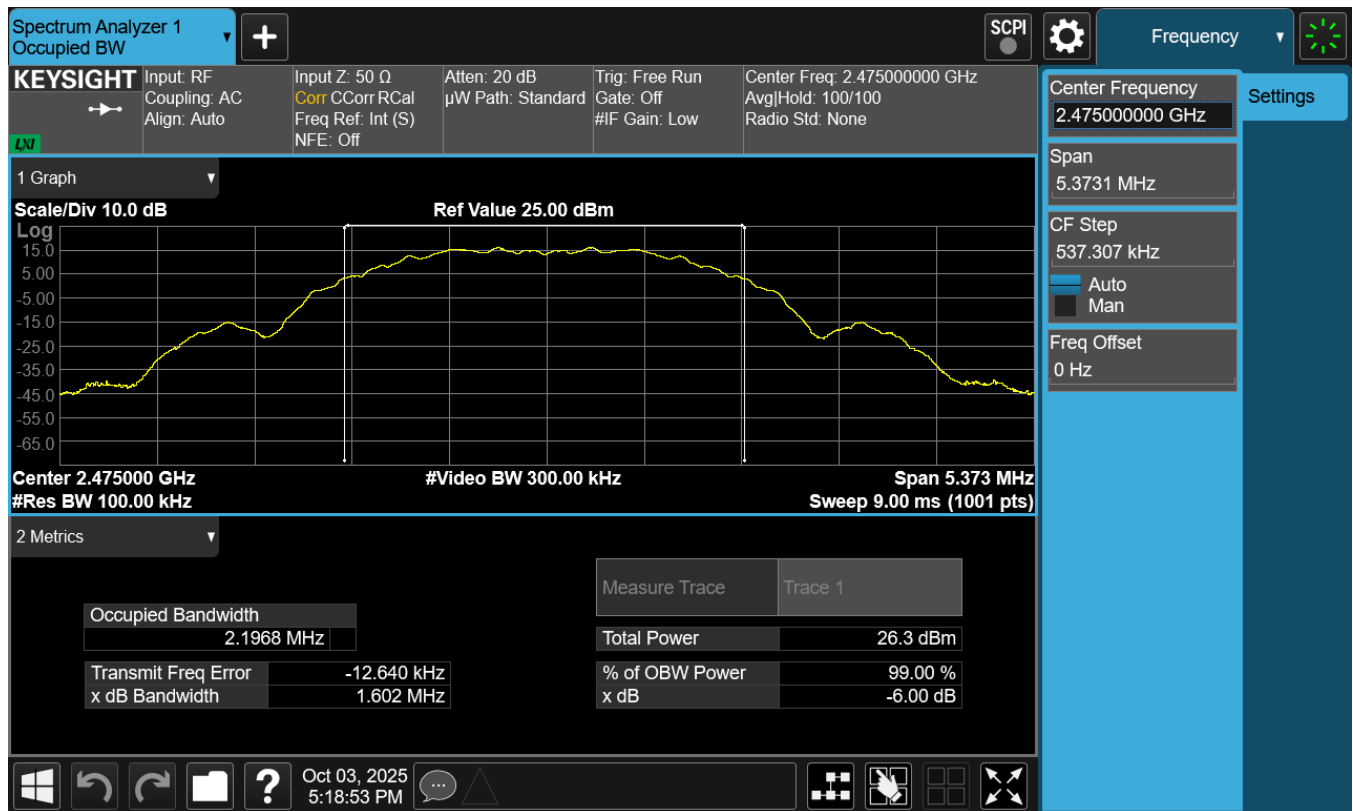
Plot 7-12. 6dB BW Antenna 1a(802.15.4, Ch. 25)
