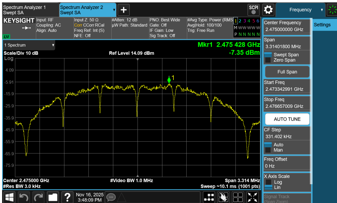
Plot 7-18. Power Spectral Density Antenna 3a (802.15.4, iPA – Ch. 25)
