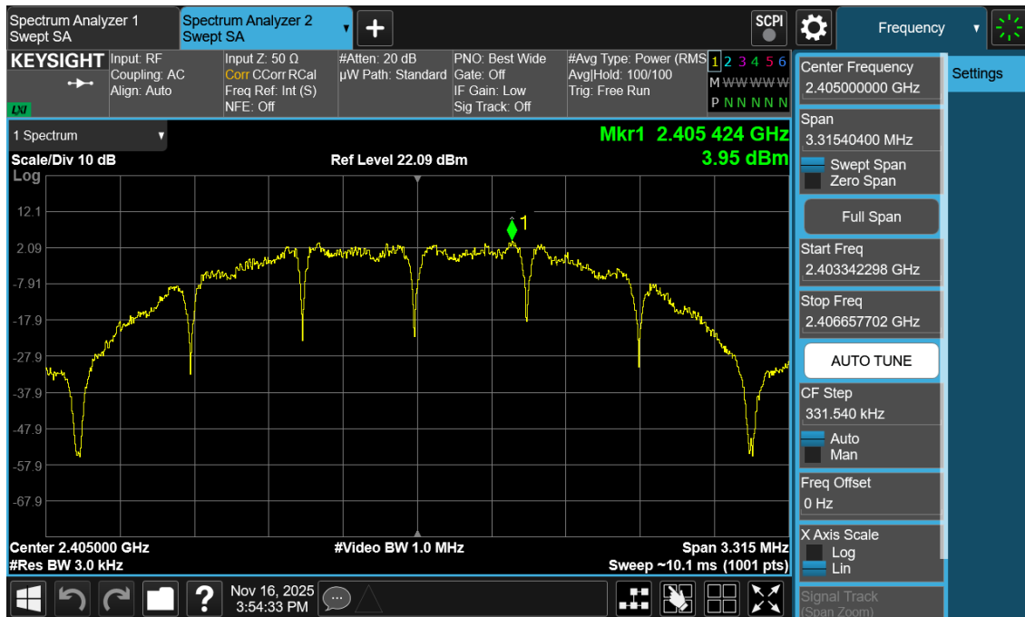
Plot 7-19. Power Spectral Density Antenna 1a (802.15.4, ePA – Ch. 11)
