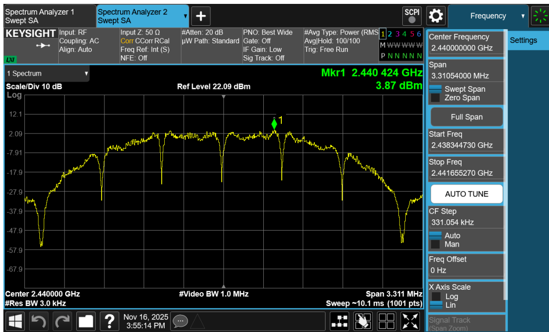
Plot 7-20. Power Spectral Density Antenna 1a (802.15.4, ePA – Ch. 18)
