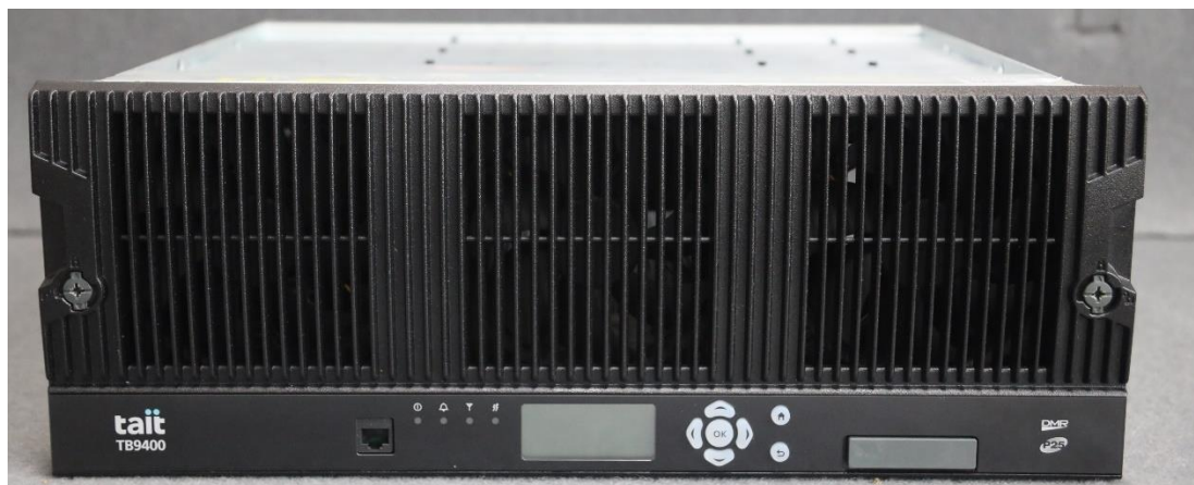
Photograph 01: Base station – Front view
