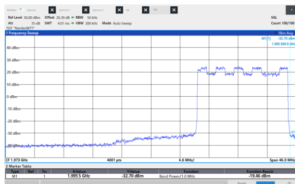
Figure 8.6-129: Conducted Spurious Emissions, High CH 1987.5 MHz, 15 MHz, 16QAM, High band edge
