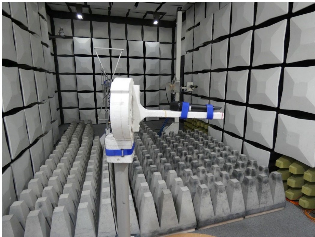
Photo 6: Setup Spurious Emissions Radiated (FAC), > 1GHz, detail view
