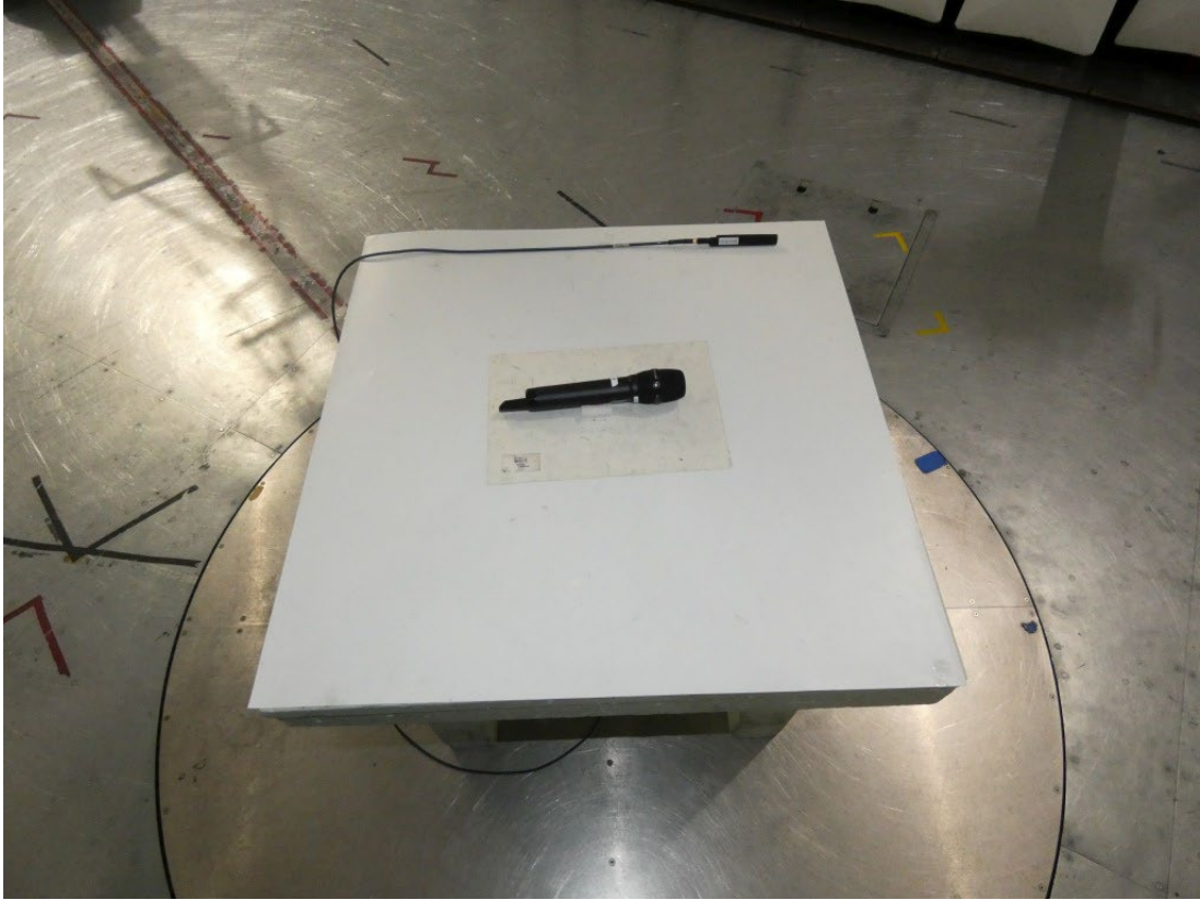
Photo 3: Setup Spurious Emissions Radiated (SAC), < 1 GHz, detail view, EUT horizontal
