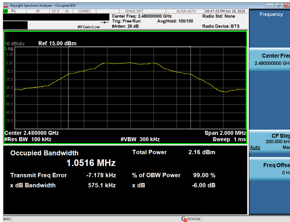
Plot 7-3. 6dB Bandwidth Plot (ANT – Ch. 79)
