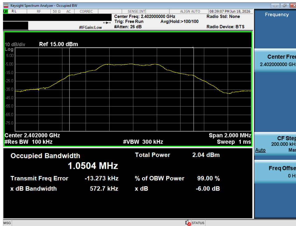
Plot 7-1. 6dB Bandwidth Plot (ANT – Ch. 1)
