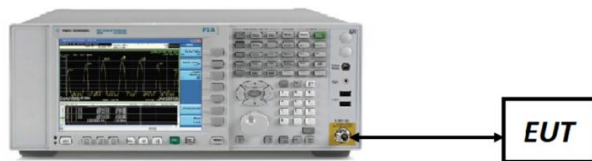
Figure 7-1. Test Instrument & Measurement Setup
