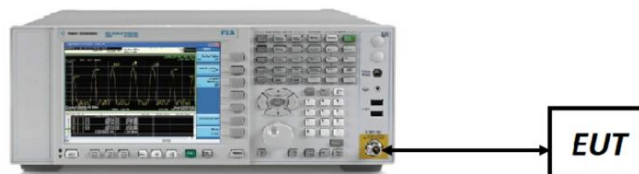
Figure 7-5. Test Instrument & Measurement Setup
