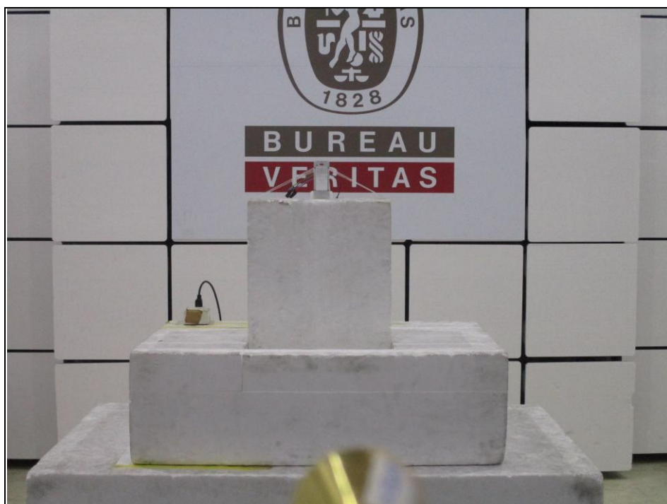
Radiated Emission Test (50GHz ~ 55GHz)
