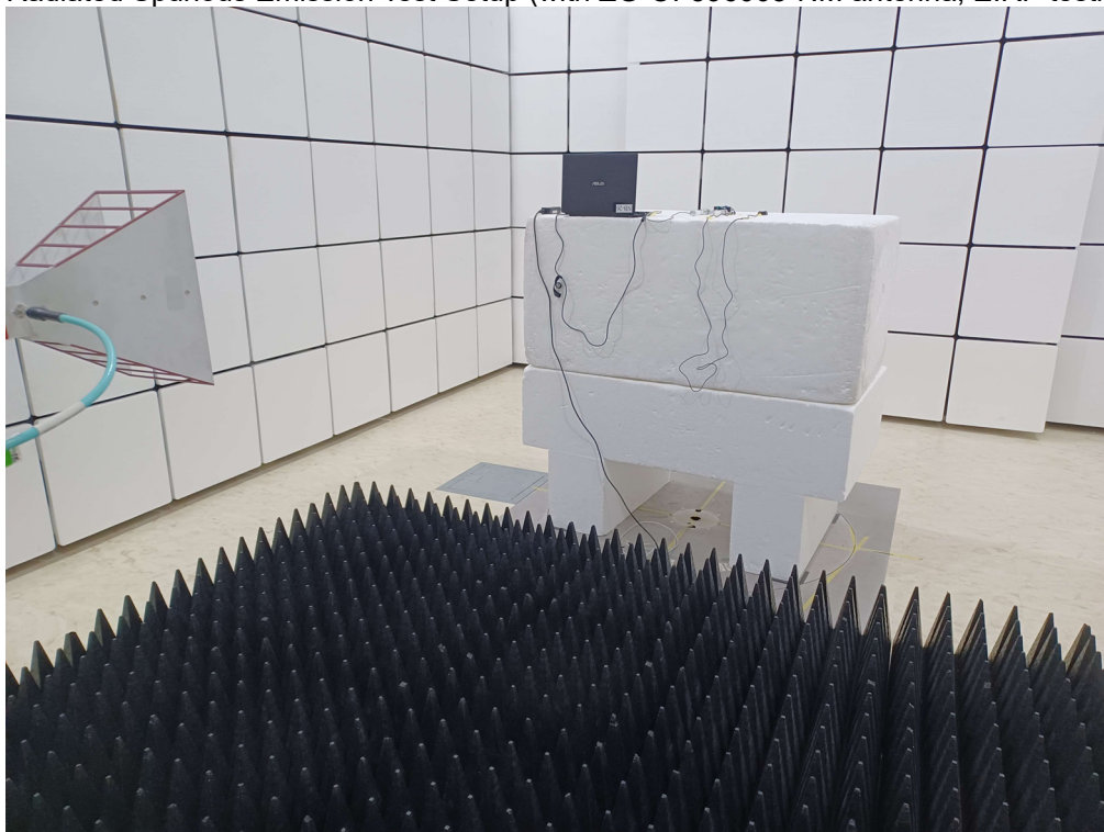
Radiated Spurious Emission Test Setup (with ZG-OI-596005-NM antenna, EIRP testing)
