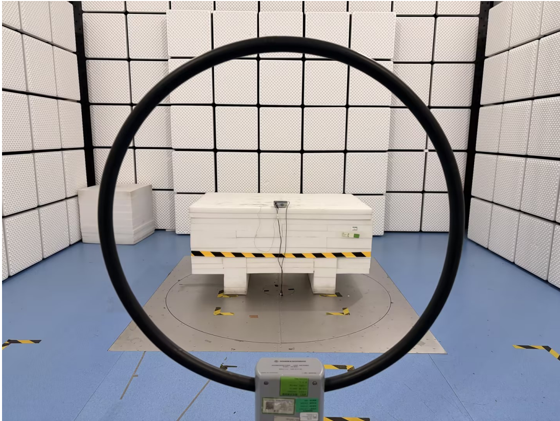
Radiation Emission - Front View (Below 1GHz)
