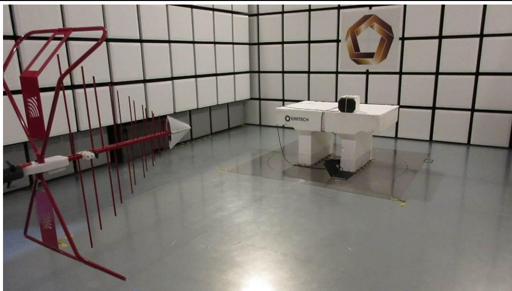
TEST SETUP PHOTO(S) - 30 MHz TO 1 GHz
