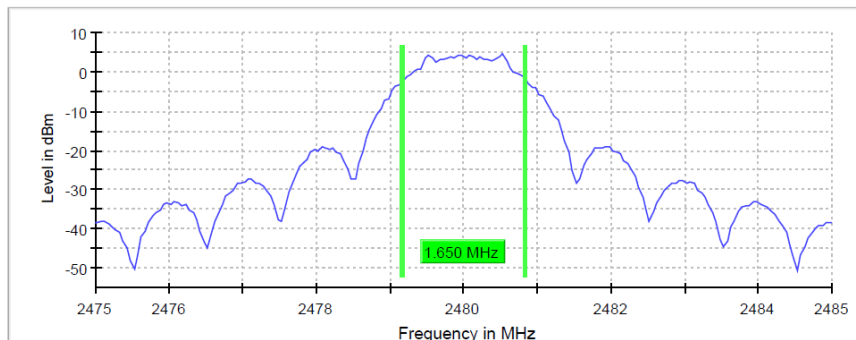
6 dB Bandwidth Plot on Configuration : Highest channel (2 480 MHz)
