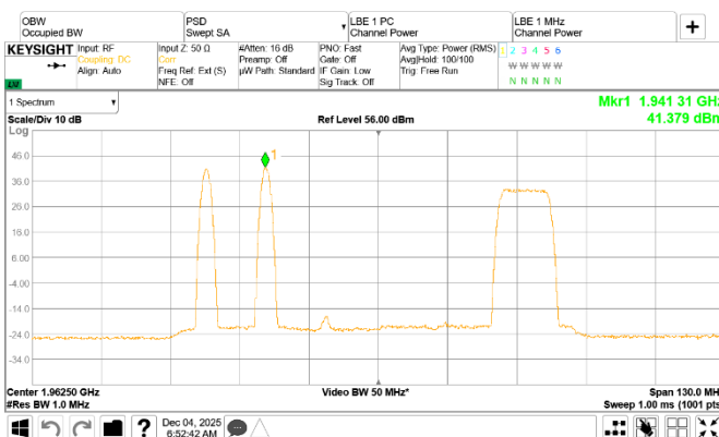
Figure 8.2-49: PSD of GSM + SA + LTE 10 MHz channel, multi-RAT operation, sample plot, Non-contiguous
