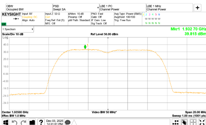
Figure 8.2-37: PSD of WCDMA + NR 5 MHz channel, multi-RAT operation, sample plot, Contiguous
