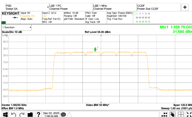
Figure 8.2-25: PSD of 6xLTE 10 MHz channel bandwidth, multi-carrier operation, sample plot, Contiguous
