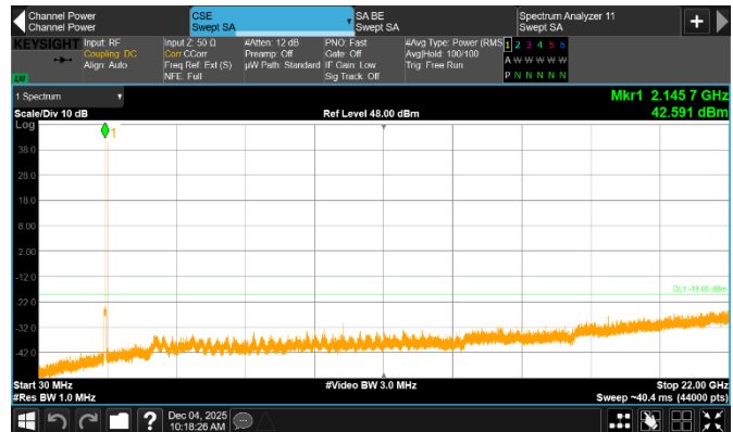
Figure 8.3-20: Conducted spurious emissions of NR 5 MHz mid channel, single carrier operation
