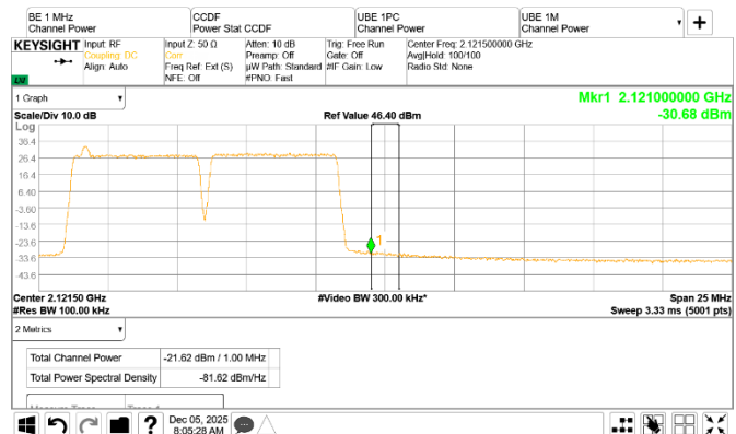
Figure 8.4-143: Conducted emission 1 MHz away at the upper frequency block edge of the lower channel
