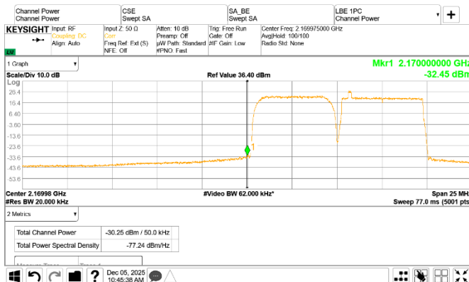
Figure 8.4-138: Conducted emission at the lower frequency block edge of the top channel
