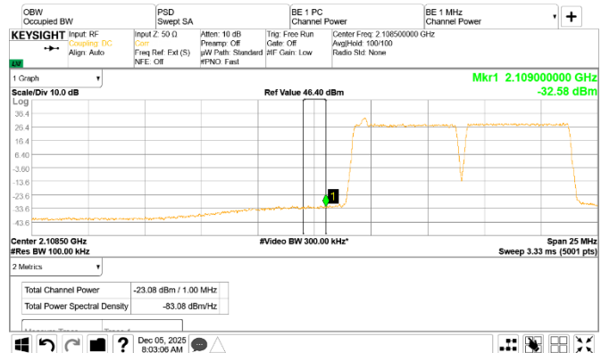
Figure 8.4-141: Conducted emission 1 MHz away from the lower band edge
