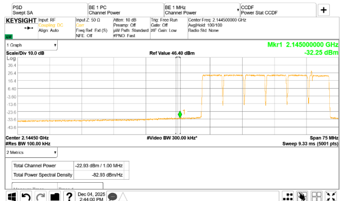
Figure 8.4-104: Conducted emission at the lower frequency block edge of the top channel
