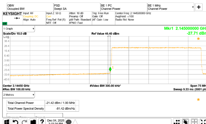
Figure 8.4-66: Conducted emission at the lower frequency block edge of the top channel
