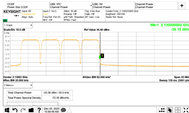
Figure 8.4-96: Conducted emission at the upper frequency block edge of the lower channel
