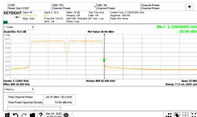
Figure 8.4-87: Conducted emission at the upper frequency block edge of the lower channel
