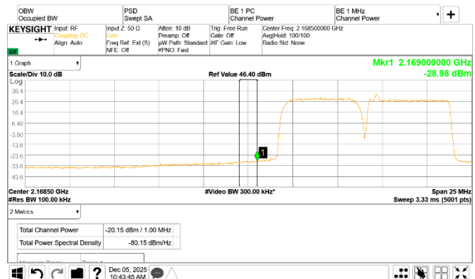
Figure 8.4-139: Conducted emission 1 MHz away at the lower frequency block edge of the top channel
