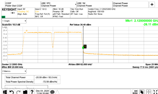
Figure 8.4-79: Conducted emission at the upper frequency block edge of the lower channel
