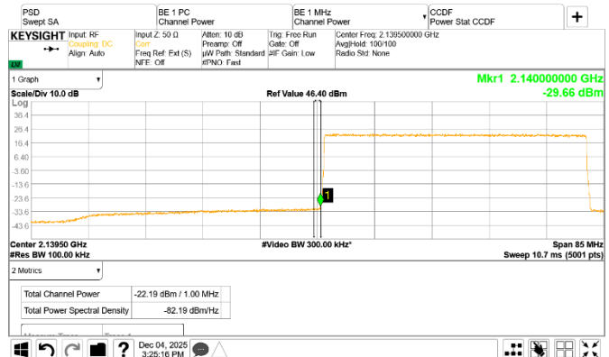
Figure 8.4-70: Conducted emission at the lower frequency block edge of the top channel
