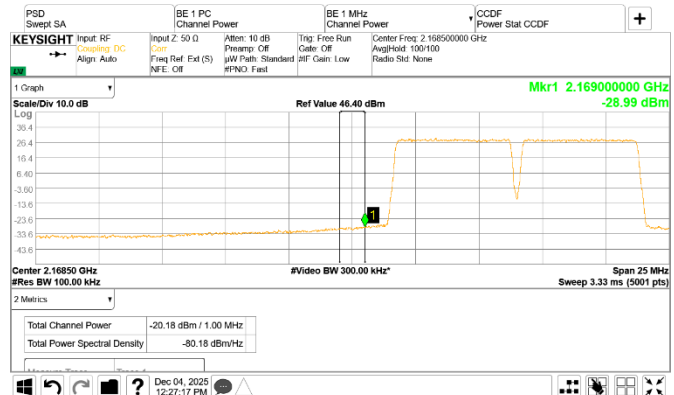
Figure 8.4-92: Conducted emission 1 MHz away at the lower frequency block edge of the top channel
