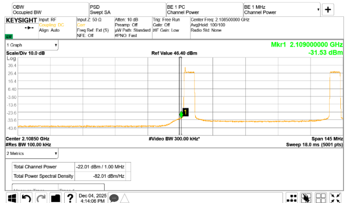
Figure 8.4-114: Conducted emission 1 MHz away from the lower band edge
