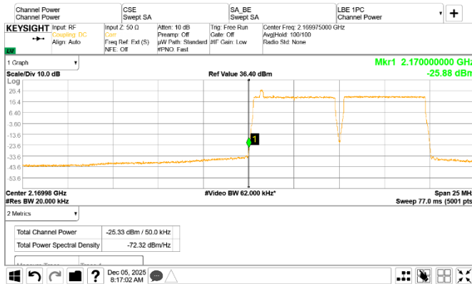
Figure 8.4-146: Conducted emission at the lower frequency block edge of the top channel
