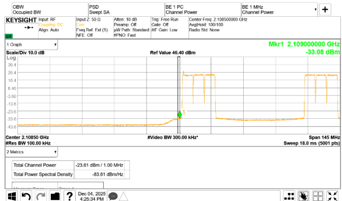
Figure 8.4-126: Conducted emission 1 MHz away from the lower band edge
