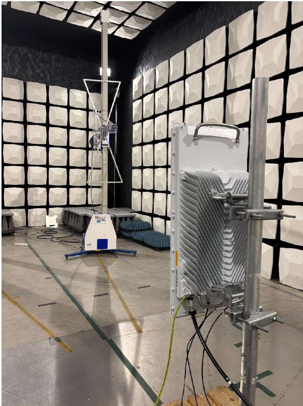
Photo of the test set-up for radiated emission 30 – 1000 MHz
