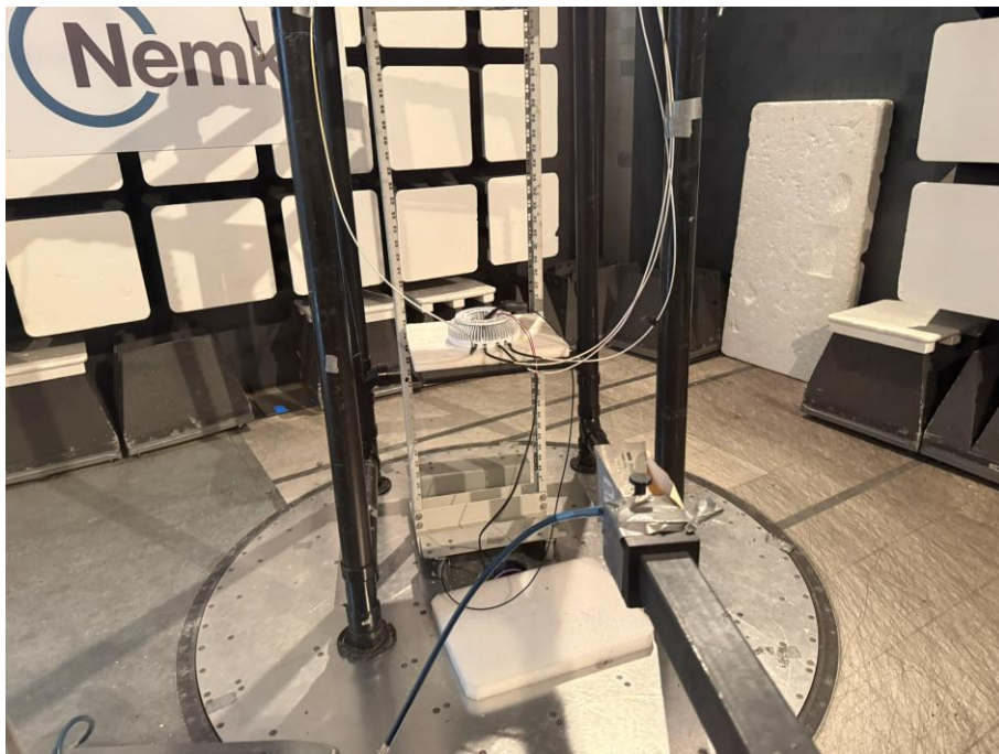
Figure 3.4-5: EUT Set-up photo for Radiated Emissions [18-26.5 GHz]
