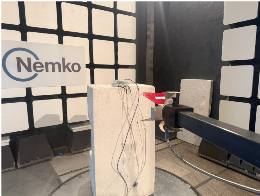
Figure 3.4-3: EUT Set-up photo for Radiated Emissions [1-10 GHz]
