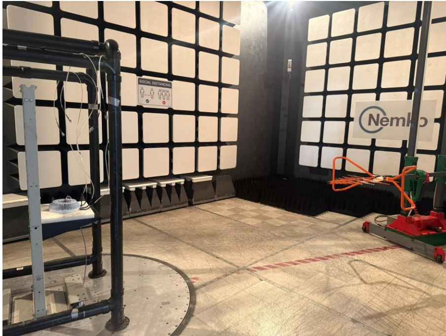
Figure 3.4-2: EUT Set-up photo for Radiated Emissions [30 MHz to 1000 MHz]
