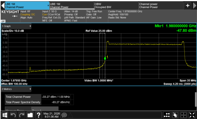
Figure 8.7-24: Conducted emission at the lower frequency block edge of the upper channel
