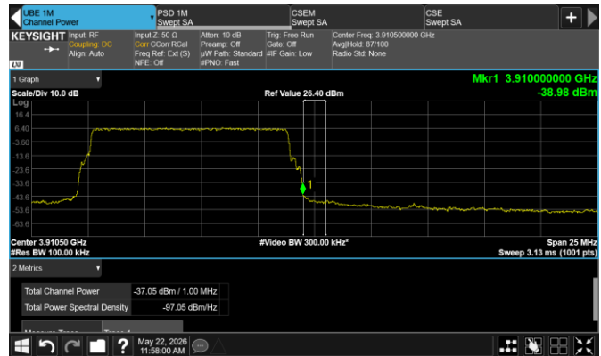
Figure 8.6-149: Conducted emission at the upper frequency block edge of the lower channel [Dot 4469 B77D – spot check evaluation]
