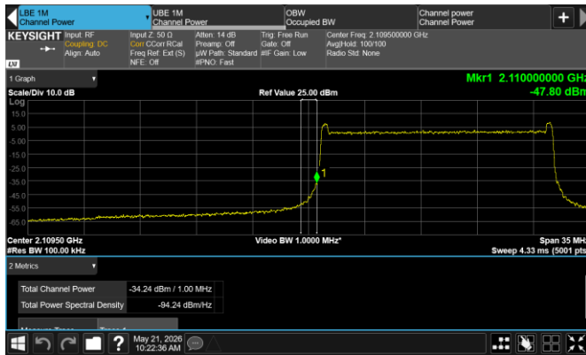
Figure 8.8-20: Conducted emission at the lower band edge
