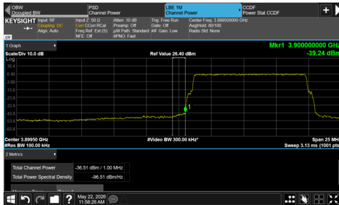
Figure 8.6-148: Conducted emission at the lower band edge [Dot 4469 B77D – spot check evaluation]
