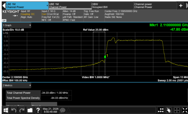
Figure 8.8-12: Conducted emission at the lower band edge
