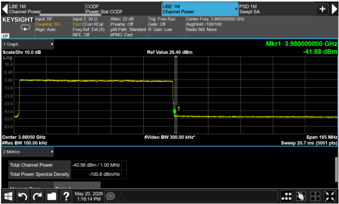
Figure 8.6-129: Conducted emission at the upper band edge
