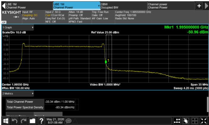
Figure 8.7-23: Conducted emission at the upper band edge
