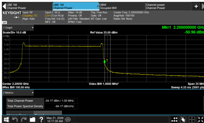
Figure 8.8-22: Conducted emission at the upper band edge
