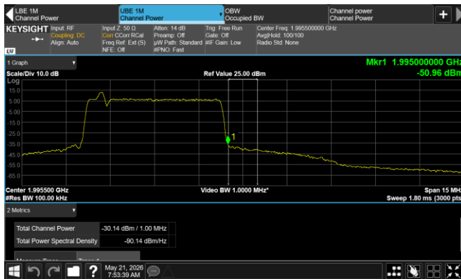
Figure 8.7-14: Conducted emission at the upper band edge
