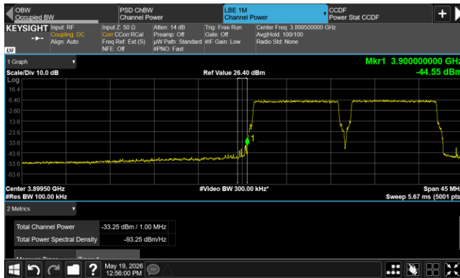
Figure 8.6-130: Conducted emission at the lower band edge
