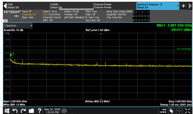
Figure 8.6-143: Conducted emission at the upper band edge [spur zoom in]
