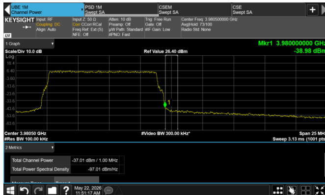
Figure 8.6-150: Conducted emission at the upper band edge [Dot 4469 B77D – spot check evaluation]
