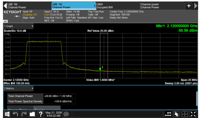
Figure 8.8-17: Conducted emission at the upper frequency block edge of the lower channel
