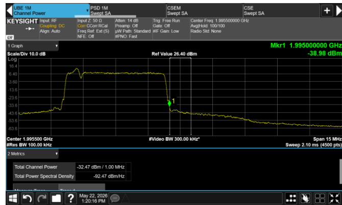
Figure 8.7-16: Conducted emission at the upper band edge for LTE 5 MHz top channel - Worst case comparison plot for model variant according to KDB 484596 Do1 Referencing Test Data
