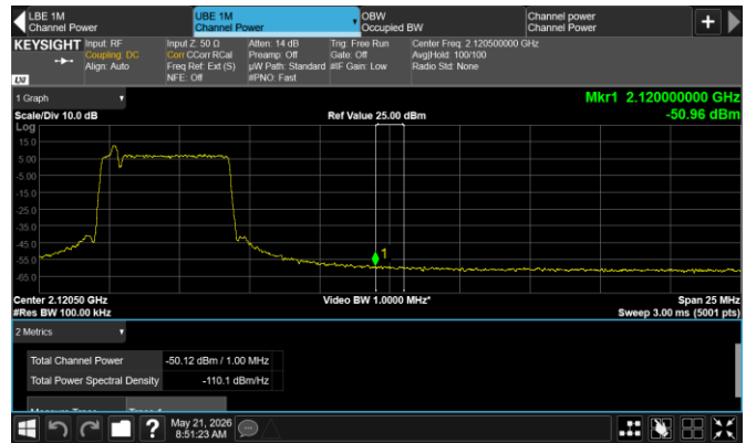
Figure 8.8-13: Conducted emission at the upper frequency block edge of the lower channel
