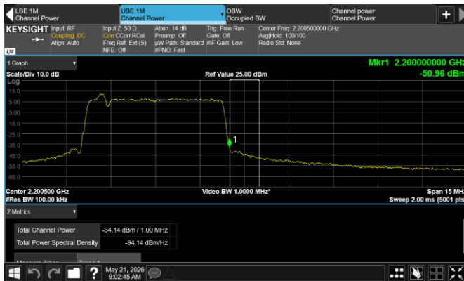
Figure 8.8-14: Conducted emission at the upper band edge
