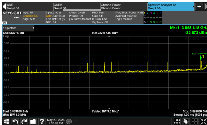
Figure 8.6-142: Conducted emission at the lower band edge [spur zoom in]
