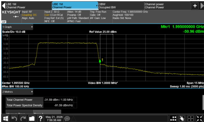
Figure 8.7-19: Conducted emission at the upper band edge
