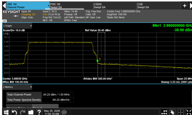
Figure 8.6-154: Conducted emission at the upper band edge [Dot 4459 B77D – spot check evaluation]
