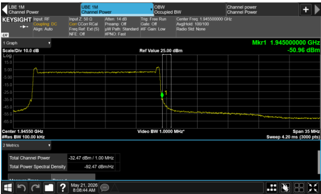
Figure 8.7-22: Conducted emission at the upper frequency block edge of the lower channel
