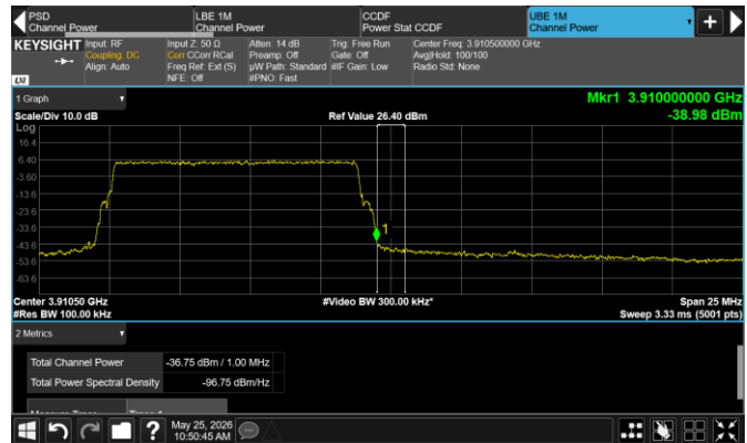
Figure 8.6-153: Conducted emission at the upper frequency block edge of the lower channel [Dot 4459 B77D – spot check evaluation]
