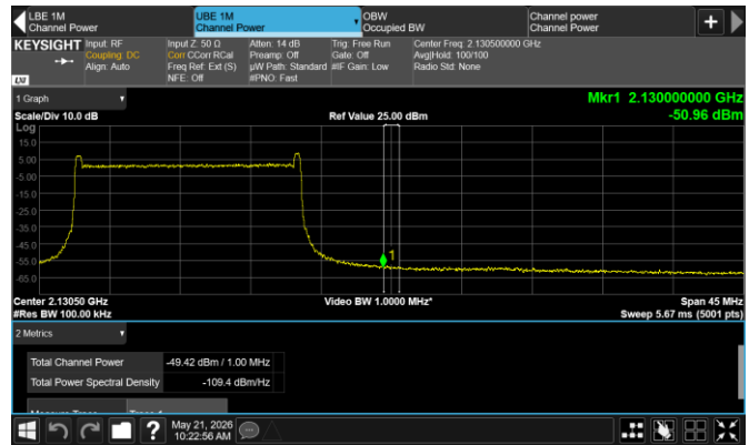
Figure 8.8-21: Conducted emission at the upper frequency block edge of the lower channel
