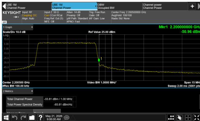
Figure 8.8-18: Conducted emission at the upper band edge
