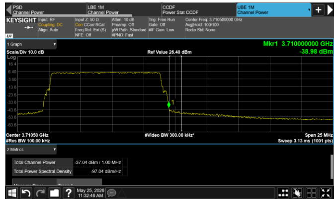
Figure 8.5-79: Conducted emission at the upper frequency block edge of the lower channel
