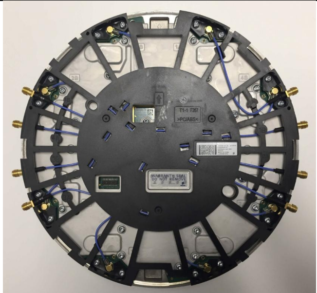
Cable carrier of referenced product Dot 4465
