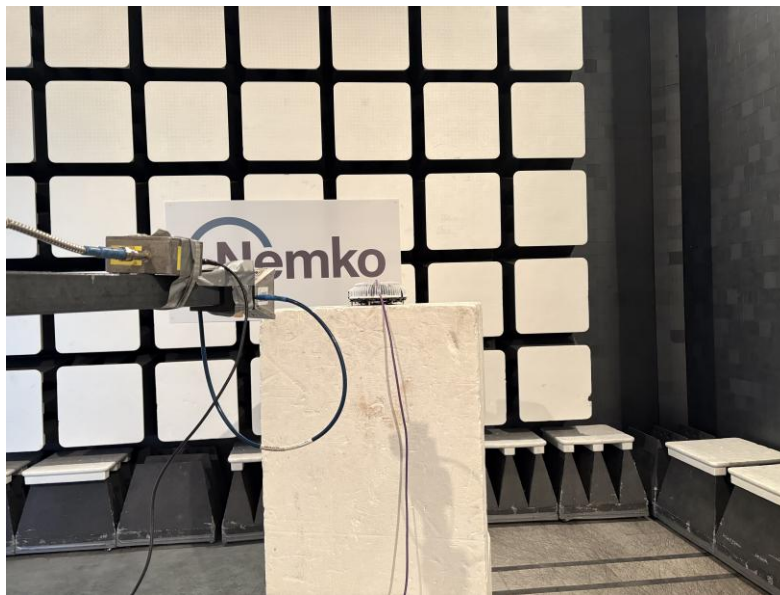
Figure 3.5-8: EUT Set-up photo for Radiated Emissions [18-40 GHz]
