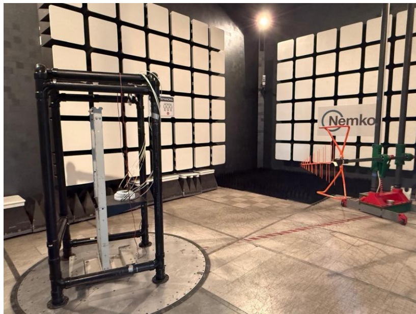
Figure 3.5-4: EUT Set-up photo for Radiated Emissions [30 MHz to 1000 MHz]
