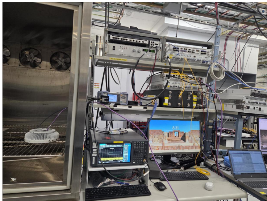
Figure 3.5-2: Set up photo for Conducted Radio Compliance Testing (thermal)
