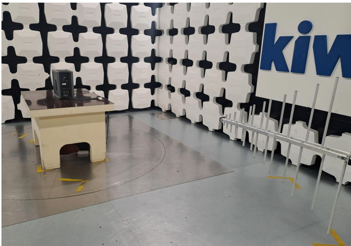
Photo 2 Photograph test setup radiated emissions 250-1000 MHz, report section 3.1
