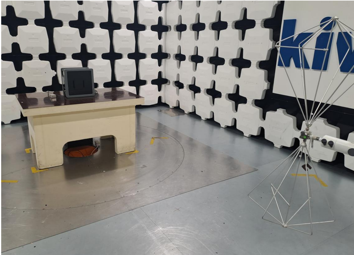
Photo 1 Photograph test setup radiated emissions 30-250 MHz, report section 3.1
